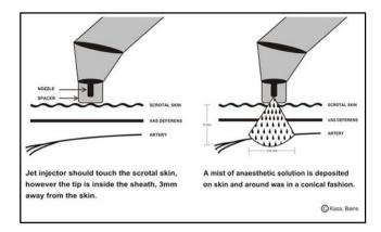
Figure 2. Jet Injector-Mechanism of Functioning
